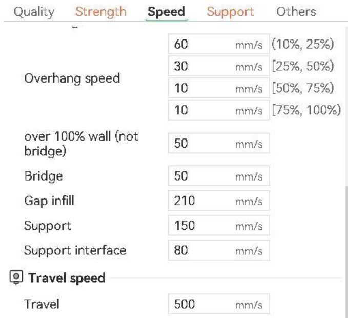
Fig. 16. Setting print speeds for the Bambu Lab printer
