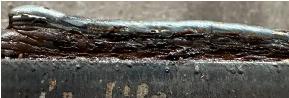
Fig. 17. A view of a vertical multi-layer wall (12.5 mm high) made by single-bead deposition, Table 3
