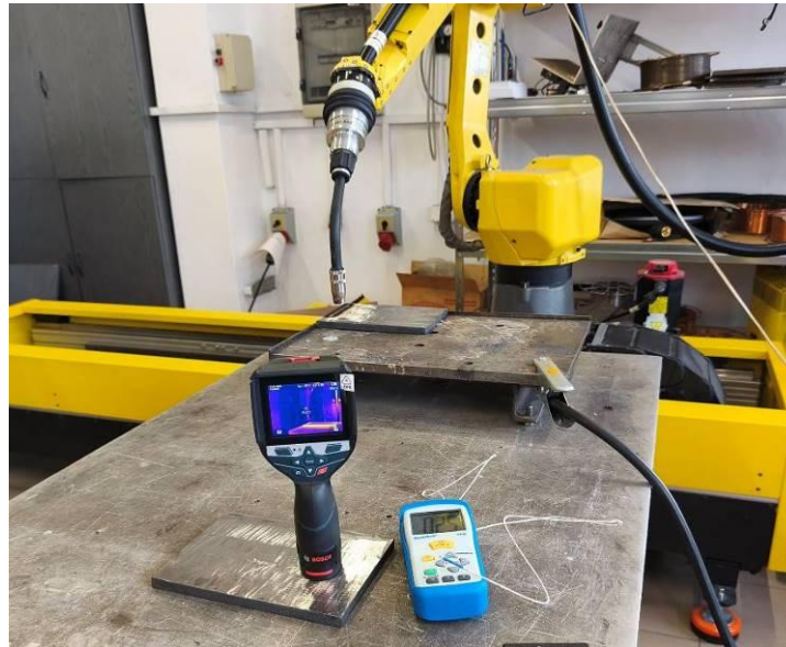
Fig. 12. A view of the experimental stand with BOSCH GTC 600C thermal imaging camera (left) and PeakTech 5110 digital thermometer with a K-type thermocouple (right)
