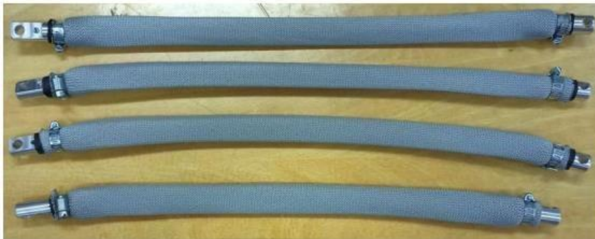
Fig. 4. Experimental pneumatic artificial muscles
