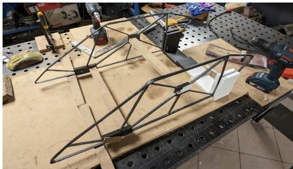
Fig. 9. Finished side parts of the bracket
