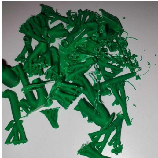
Fig. 6. Material removed after post-processing
