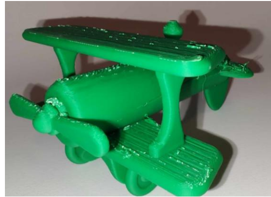
Fig. 5. 3D printed ABS part (airplane)
