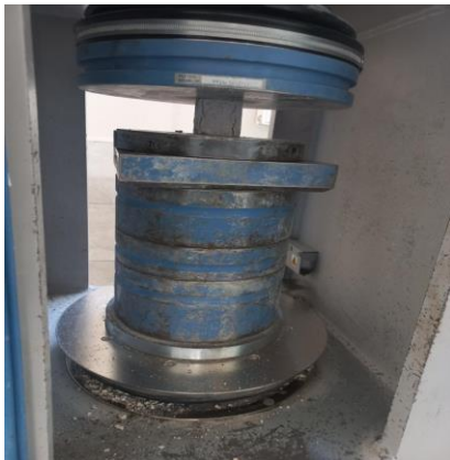
Fig. 3. Compressive strength tests for mortar samples
