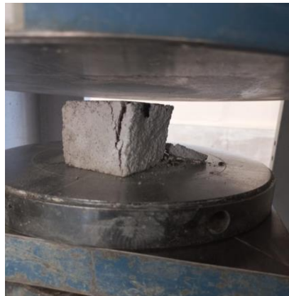
Fig. 3. Compressive strength tests for mortar samples
